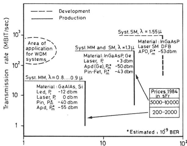
Fig. 9 Optoelectronic devices for digital fiber transmission systems
