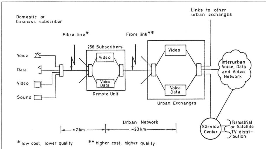
Fig. 6 Wideband ISDN scenario for voice, data and video services after 1990
