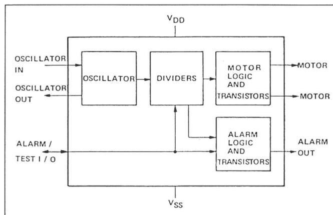
Fig. 1 Block diagram of a conventional clock device (8 pin)
