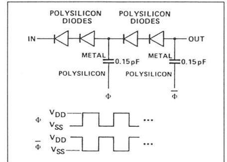
Fig. 5 Two stages of the voltage multiplier
