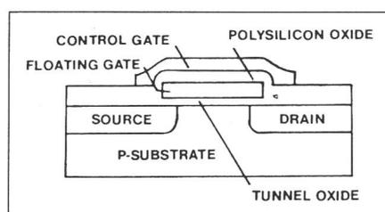
Fig. 1 Memory transistor
