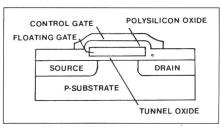
Fig. 1 Memory transistor
