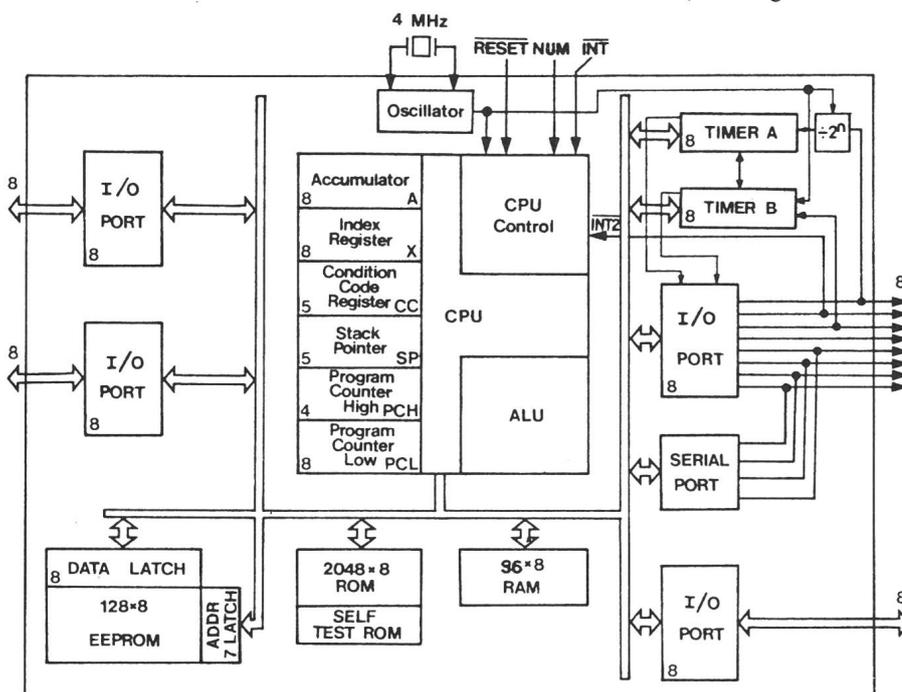
Fig. 4 Microcomputer blockdiagram (MC 6805 K2)
