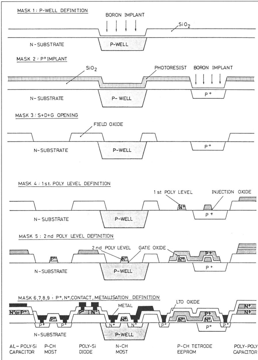
Fig. 1 1.5 V 10 mask CMOS process
