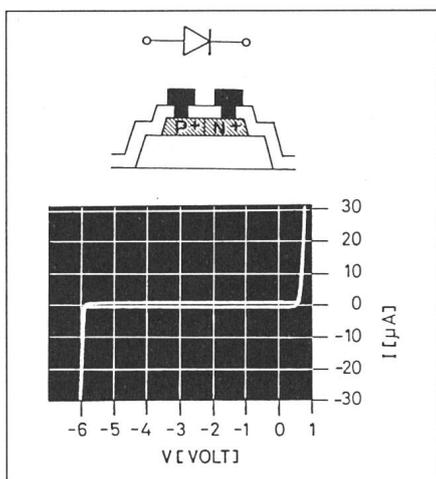
Fig. 2 I-V Characteristic of a Poly-Si Diode
