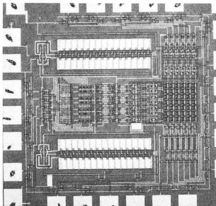
Fig. 14 Microphotograph of a  $7 \times 6$  bit EEPROM
