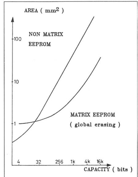
Fig. 3 Non-matrix and matrix EEPROM, comparison of area
