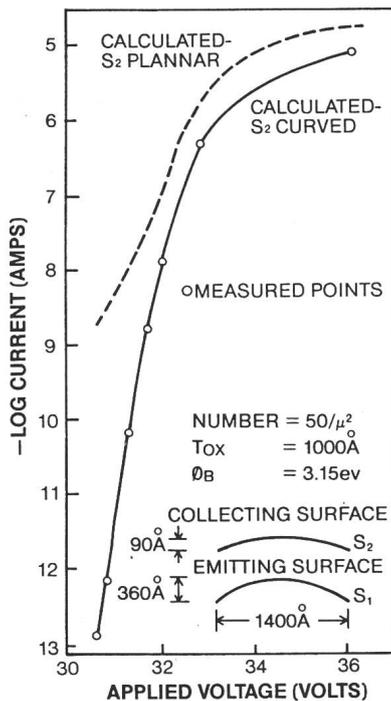
Fig. 5 Reverse Tunneling Characteristics for Textured Poly Floating Gate Technology
