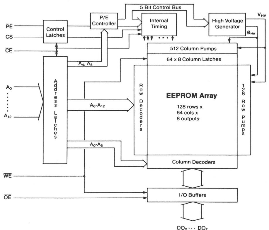
Fig. 9 Functional Block Diagram of IMS 3630
