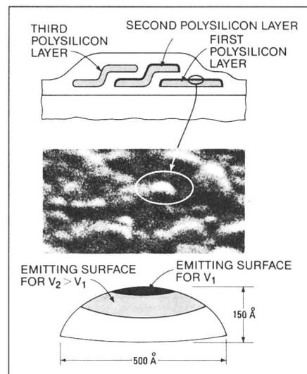
Fig. 3 64 K EEPROM: Floating Gate Technology with Textured Poly
