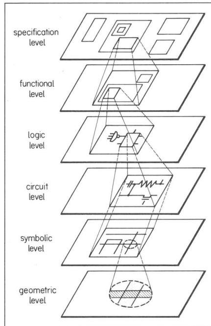
Fig. 5 Abstraction levels of VLSI design process
