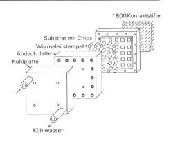
Fig. 11 Thermal Conduction Module (TCM)
