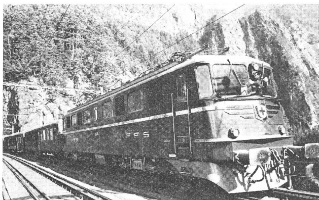
Fig. 9 Gotthardlokomotive Co'Co' Ae 6/6 der SBB (1953...1966)
