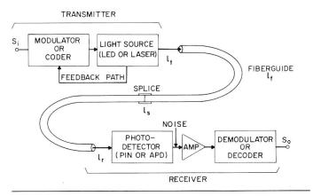
Fig. 1 Generic block diagram of a fiberguide transmission system
