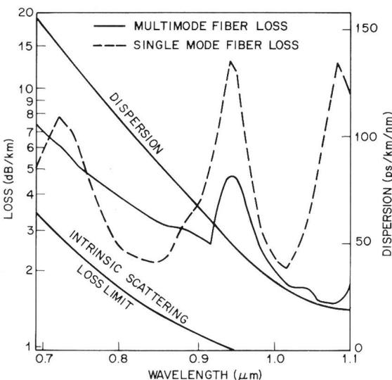
Fig. 7 Typical loss versus wavelength characteristics of a multimode and a single-mode fiberguide [29]
