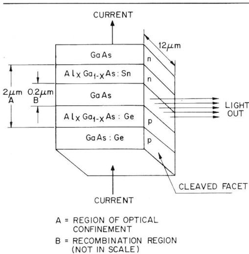
Fig. 2 Schematic diagram of an AlGaAs double-heterostructure laser
