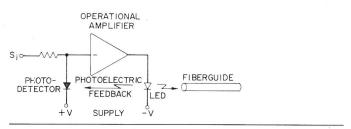
Fig. 5 Schematic of LED transmitter circuit with photoelectric feedback
