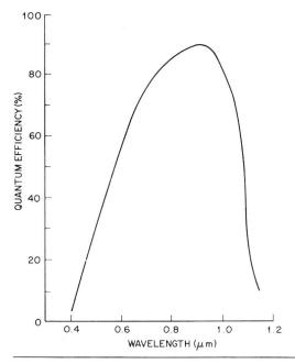
Fig. 9 Quantum efficiency as a function of wavelength for a PIN Photodetector with wide depletion regions, optimized for maximum response at 0,9 μm [18]
