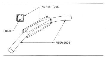
Fig. 8 The loose tube splice
