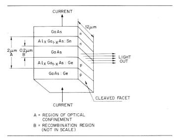
Fig. 2 Schematic diagram of an AlGaAs double-heterostructure laser
