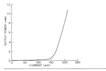
Fig. 3 Typical curve of radiated power of an AlGaAs double-heterostructure laser as a function of current
