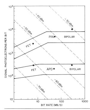
Fig. 10 Minimum primary photoelectrons generated at the photodetector per bit interval of incoming information as a function of bit rate, for a fixed error probability of 10<sup>-9</sup> [19]
