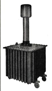
Prüttransformator 50/100/200kV 40kV A
