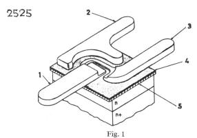
MIS-Transistor in Beam-lead-Technik
