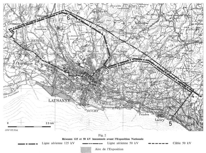
1 Station 125/50/6 kV Banlieue-Ouest; 2 Station 50/6 kV Sébeillon; 3 Usine et station 125/50/6 kV Pierre-de-Plan; 4 Poste de couplage 50 kV Bois-de-la-Chaux; 5 Station 50/6 kV Lutry; 6 Station 220/125 kV Romanel (EOS)
