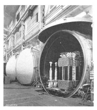
${\bf Fig.} \ \ 6$   ${\bf Vakuum\hbox{-}Ofen\hbox{-}Anlage \ mit\ horizontaler} \ \ {\bf Beschickung}$
