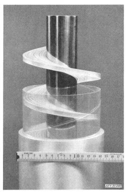
${\bf Fig.~3} \\ {\bf Starkes~Antennenspeise kabel~mit~Bandwendelisolation}$
