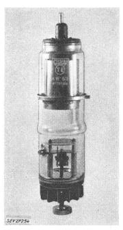
$\begin{array}{c} {\rm Fig.~20} \\ {\rm \bf Excitron~AR63} \\ {\rm f\"{u}r~12~000~V~~5~A~Dauerbetrieb} \end{array}$
