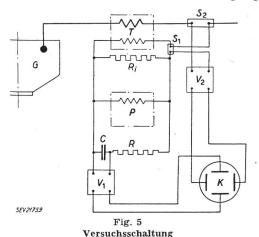
G T Ri PMutator Stromwandler Widerstand
