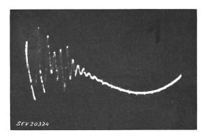
$\begin{array}{c} {\rm Fig.~3} \\ {\rm Beginn~des~Impulses~nach~Passieren~des~Hochpassfilters} \\ {\rm Zeitmarke}\,{=}\,1\,\mu s \end{array}$
