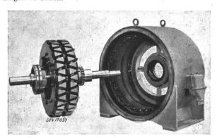
Fig. 1 50-kW-Gruppe 1000 V; 400...900 Hz; n = 1200...2700/min
