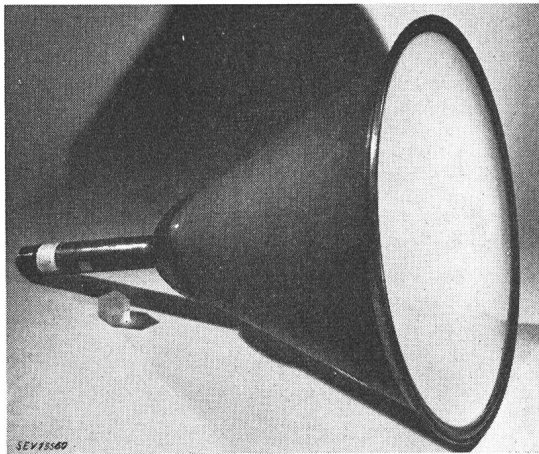
Fig. 20 16-inch Kinescope with Metal Wall
