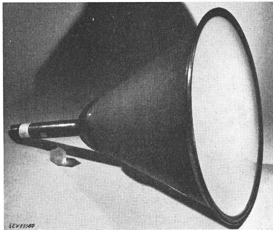
Fig. 20 16-inch Kinescope with Metal Wall
