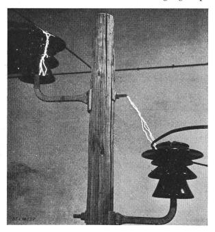
${\bf Fig.~9} \\ {\bf 50\text{-}\%\text{-}Stoss\"{u}berschlag}, \\ {\bf -390~kV} \ ({\tt kleinster~Wert})$
