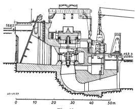
$\label{eq:Fig. 11 c.} \text{Wheeler-Damm, Ala. 1936. } H = 16.2 \text{ m; } 4(8) \times 36000 \text{ kVA.}$
