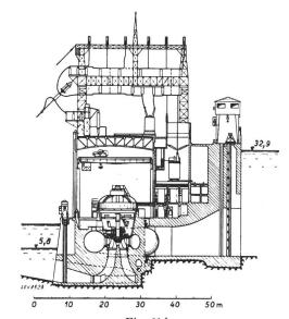
Fig. 11 b. Conowingo, Md. 1928. H = 27.1 m;  $7(10) \times 40000$  kVA.
