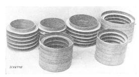
${\rm Fig.~3.} \\ {\rm Aus~~ {}^{\circ} Transformer board {}^{\circ}~ gezogene~ Winkelringe.}$
