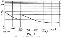
$\begin{array}{c} \textbf{Empfindlichkeitskurve.} \\ U_1 = \textbf{F} \ (f) \, ; \ P = 50 \ \ \text{mW} \, ; \ f_{\,\text{m}} = 400 \ \ \text{Hz} \, ; \ m = 30 \ \%. \end{array}$
