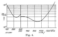
Kurve der Spiegelfrequenzempfindlichkeit.  $\frac{U_{\bullet}}{U_{1}} = F(f); P = 50 \text{ mW}; f_{m} = 400 \text{ Hz}; m = 30\%.$
