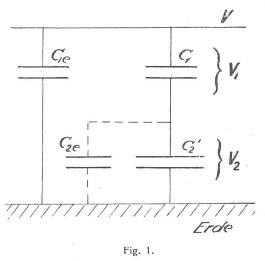
$$\frac{V_1}{V_2} = \frac{C_2}{C_1}$$
