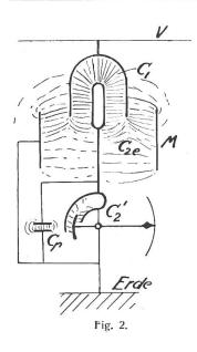
$$V_2 = V_1 \frac{C_1}{C_2}$$
