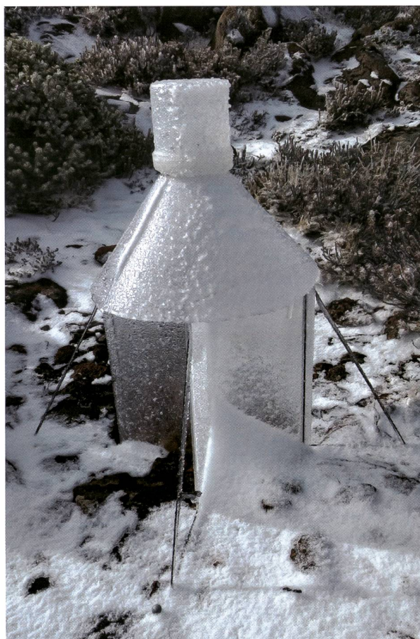
Figure 2. Basic Alpine Malaise Trap deployed on kunanyi/Mount Wellington, Hobart (Fig 1.), Tasmania, 2017.
