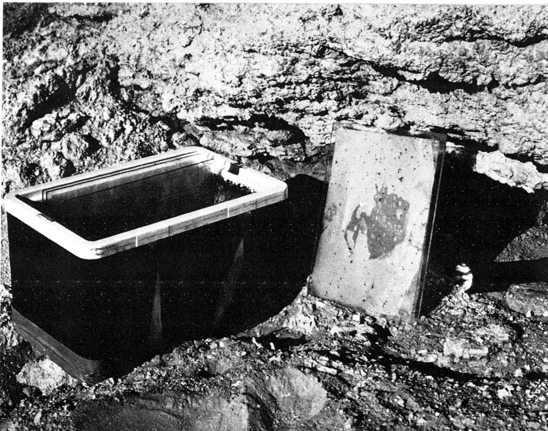
Fig. 1: View of sampling site in a natural desert biotope. Note the torch behind the plastic plate producing diffuse light on oil-coated surfaces and attracting sandflies from the neighbourhood. The coolbox is equipped for transporting plastic plates.
