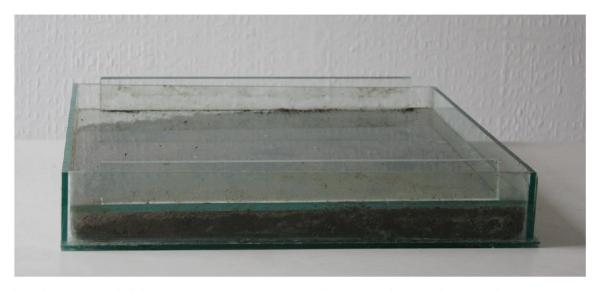
Fig. 1. Terrarium filled with soil and with the lid on. Base dimensions: 360 mm x 325 mm x 60 mm, glass thickness 4.6 mm. Lid dimensions: base 346 mm x 311 mm, glass thickness 6.2 mm; handles: 301 mm x 29 mm, glass thickness 8.4 mm.
