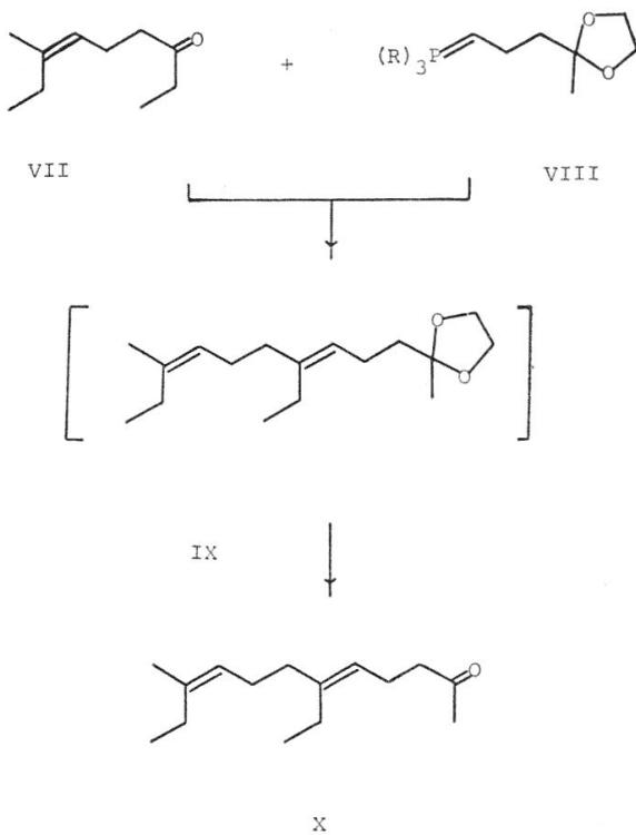
The ketal phosphonium salt VIII was prepared quantitatively from 5-iodo-2-pentanone (obtainable by NaI/acetone treatment of commercially available 5-chloro-2-pentanone) by ketalization and subsequent reaction with triphenylphosphine in boiling benzene. The stable crystalline salt VIII readily separated from this medium.
