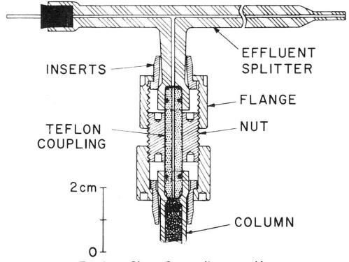
Fig. 6. — Glass effluent splitter assembly.
