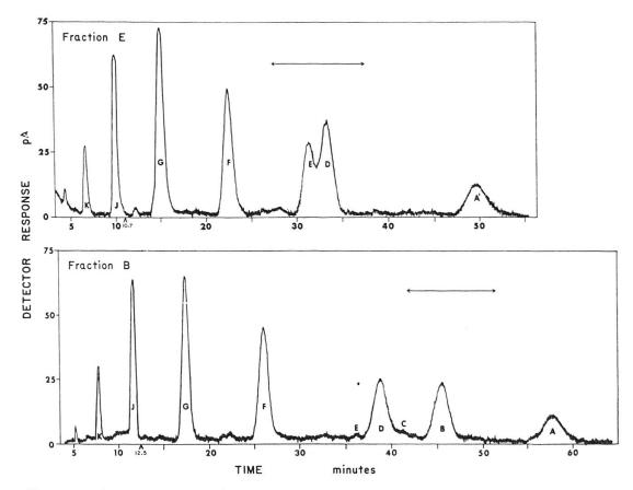
Fig. 3. — Chromatograms of Fraction E and of Fraction B (each 0.5 μg). These fractions had been isolated by micropreparative glc of the nearly pure preparation of the second Cecropia batch and trapped after passing through the argon detector at 190° C.
