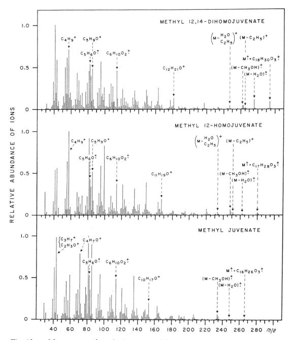
Fig. 12. — Mass spectra of synthetic compound I and natural compounds II and III. Elemental compositions were determined by high-resolution mass spectrometry and have been indicated in the diagrams for a number of selected ions; the abundance of these ions amounts to 75% or more of that represented by the particular bar.
