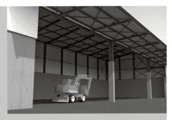
as snow can be moved by the wind and slide from the roof onto the canopy below. The snow and wind loads are carried by the girders, which are designed as trussed beams. Special attention was paid to the use of compact components and simple assembly.
