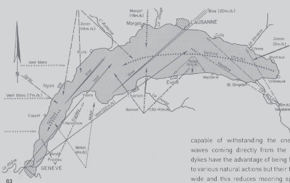
The objective of this project is to double the capacity of the Geneva marina since all the marinas on Lake Geneva are currently saturated. The future port would be protected by two dykes. Waves are the main activity to be considered when sizing a dyke. Waves are primarily induced by various winds blowing on Lake Geneva. The maximum wave height was defined as 1.7m. A "gravity" type dyke at the north with a solid structure should be
