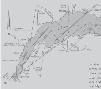
The objective of this project is to double the capacity of the Geneva marina since all the marinas on Lake Geneva are currently saturated. The future port would be protected by two dykes. Waves are the main activity to be considered when sizing a dyke. Waves are primarily induced by various winds blowing on Lake Geneva. The maximum wave height was defined as 1.7 m. A "gravity" type dyke at the north with a solid structure should be
