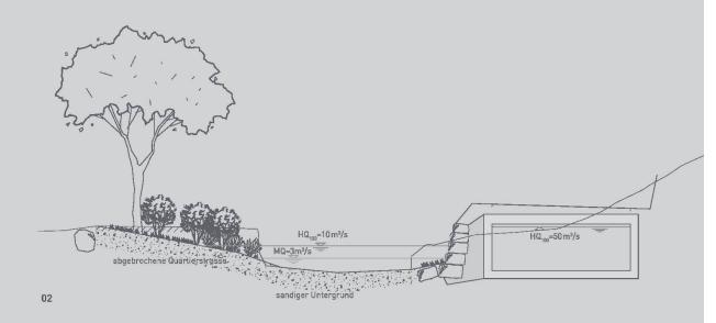
The Seeweren stream flows out of Lake Lauerz, traverses the village of Seewen and joins the Muota river about 2.4 km further downstream. Flood protection and the ecological condition of the Seeweren are inadequate. The stream is incapable of not breaking its banks when flooding attaining 22 m³/s occurs, which is the case every two years. The Seeweren is fully channelled in contradiction to present hydraulic engineering philosophy.
