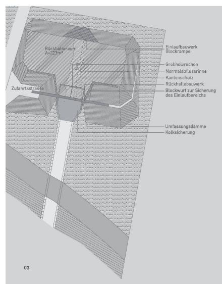
The Sylerbach culvert under the cantonal road in the Lütschine valley is too narrow. Flood waters bring floating debris that blocks the opening to such an extent that flooding occurs and the cantonal road must be closed. The planned refurbishment therefore intends to develop a flood protection concept to alleviate the situation.
