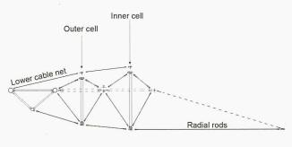
Cross section along the vertical struts
