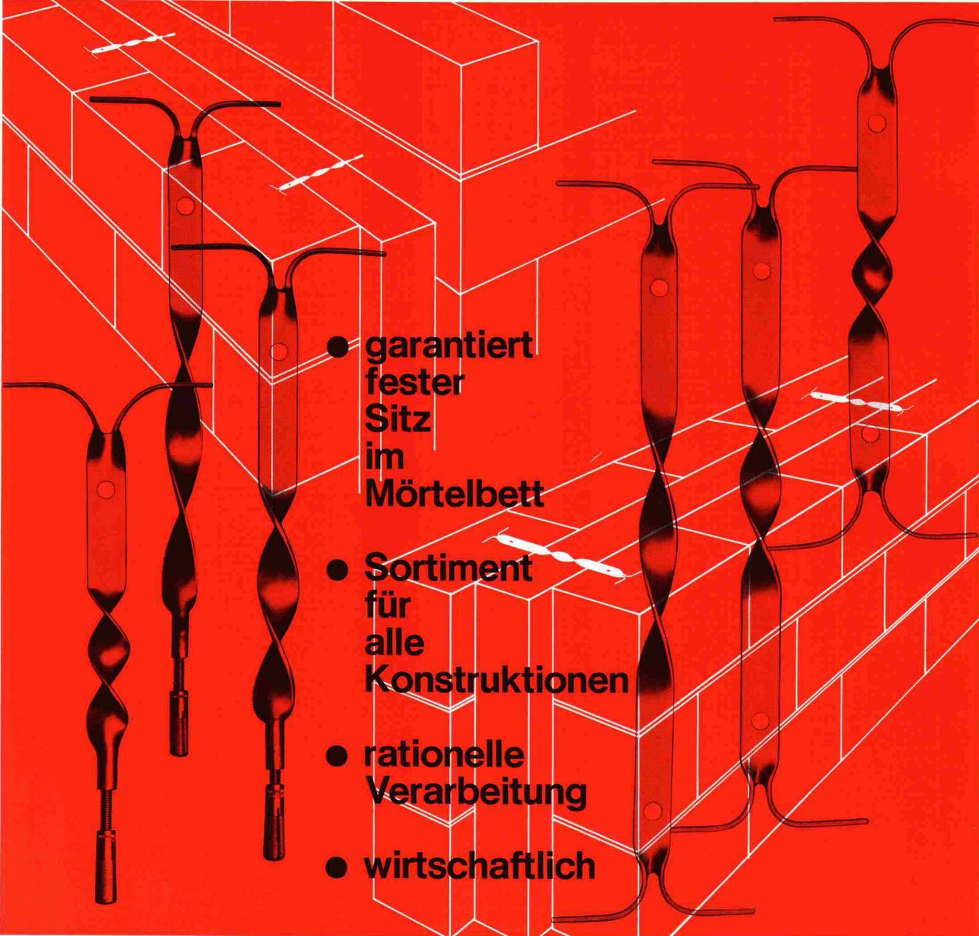
The image shows a technical drawing of spiral anchors (Spiralanker) used for securing double-shell masonry (Zweischalenmauerwerk). The drawing is set against a red background with white lines representing the brickwork and mortar joints. Several anchors are shown in different orientations and positions, illustrating their use in various construction scenarios. The anchors have a twisted, spiral design and a hook-like end for easy installation.
