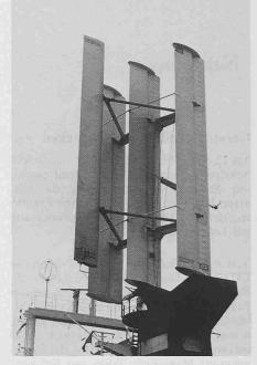
been recorded by the shipowners. On several occasions the wingsail had been used as a thruster in dockside manœuvring saving the use of tugs costing up to £ 1000 a time.
