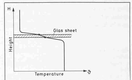
Fig. 24. Temperature gradient through the glass sheet as an insulation layer for infrared reradiation.
