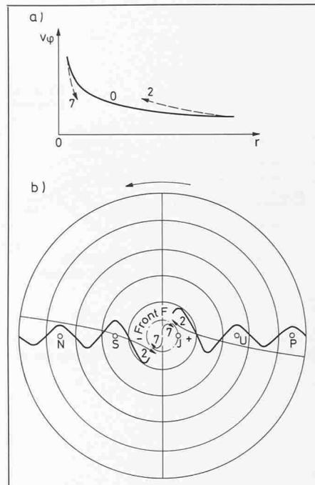
Fig. 31 (right). a) Rotating pattern of the primordial nebula disk (curve 0 for  $r^{1/2}v_\phi = \text{const}$ ) and variations of swirl velocities of the surface winds 2 and 7 (according to  $rv = \text{const}$ )
