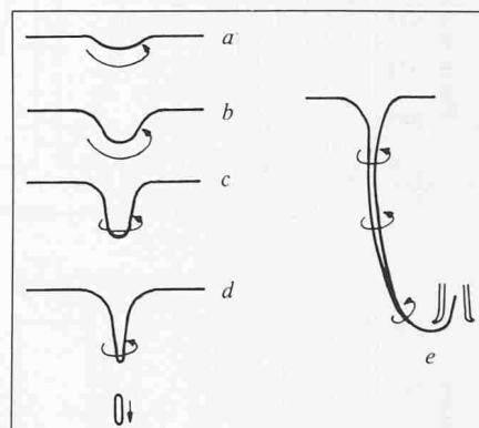
Fig. 7. Stages in development of an air-entraining vortex (Denny)
