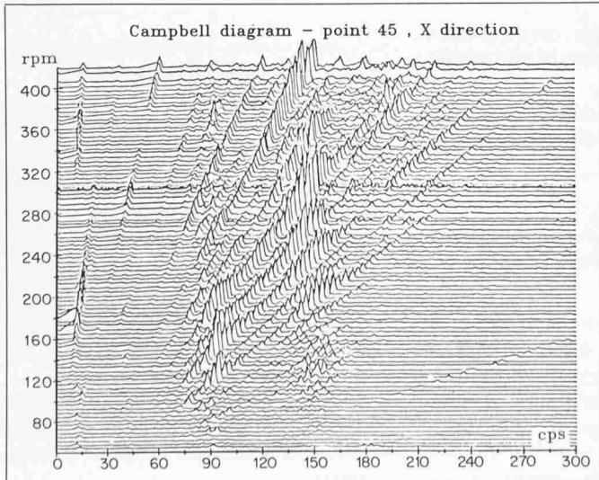
Fig. 3. Order Ratio diagram related to the extrusion press
