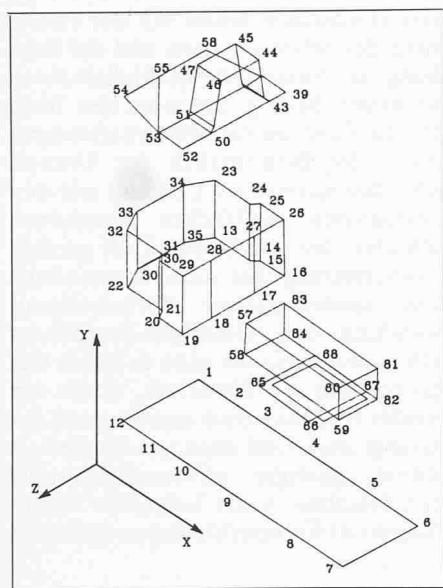
Fig. 1. Exploded view of an extrusion press
