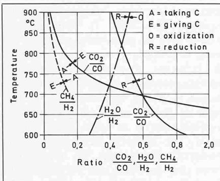
Fig. 54. Equilibrium under technical condition at a pressure of 1 bar for the gas components CO; H<sub>2</sub>, CH<sub>4</sub> and CO<sub>2</sub> (D. Dioszeghy and M.V.R. Ungarn, 1970)
