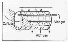
Trommelsieb. Schema (Firma Alpha, Ni-
