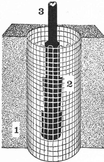
1 = Schnitt Beton    2 = Beton-Drahtkern
