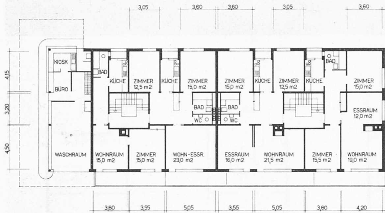
Block A, Erdgeschoss 1:400
