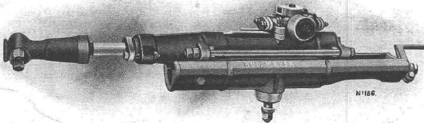
Schwere Tunnelbohrmaschine System Meyer
