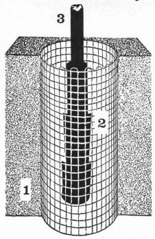
1 = Schnitt Beton 2 = Beton-Drahtkern
