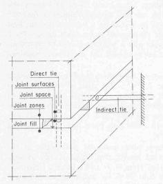
Fig. 1. Structural joint between precast units. Characteristic parts
