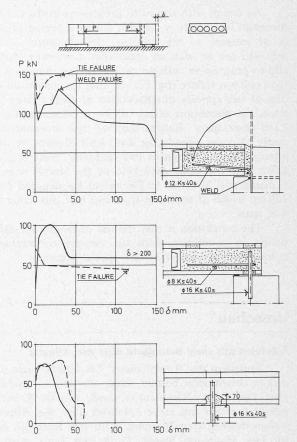
Fig. 18. Horizontal displacements at various type of supports versus an applied horizontal load. The tests are to be regarded as pilot investigations in order to give an idea of the ductility of the tie arrangement. Tests: AB Strängbetong
