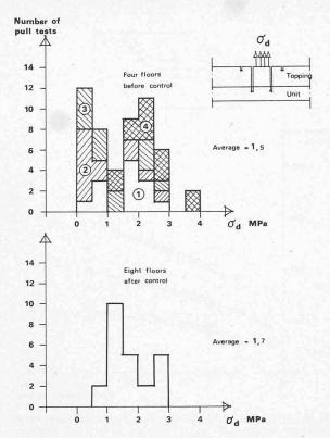
Fig. 5. Tensile bond strength at the interface between TT-slabs and concrete topping measured during construction of an 80 000 m² hospital building. The tests were made by pull up of cylinder cores using a method developed at the Swedish Cement and Concrete Institute. Low results were measured at two floors on the slab part of the TT-section. Complementary measurements showed, however, that the corresponding bond above the TT-beams was high
