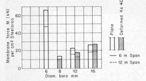
Fig. 17. Calculated maximum membrane force when loss of a central support assuming the ultimate elongation values according to fig. 16. The calculation is made for the floor spans 6 and 12 m
