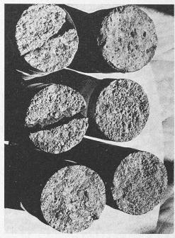
Fig. 6. Examples of rupture surfaces at interface from the tests according to fig. 5. Upwards left ice christals and upwards right a sediment layer from curing can be seen. Insufficient compaction at interface is shown by the two central surfaces and the bottom ones examplify good bond
