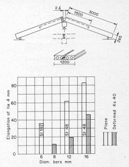
Fig. 16. Elongation of different type tie bars at a support joint, the ties being anchored in the longitudinal grouted joints between 27 cm deep and 60 cm wide hollow core prestressed slabs. In all the cases represented in this diagram the end anchor was capable of anchoring the full tensile strength of the bar
