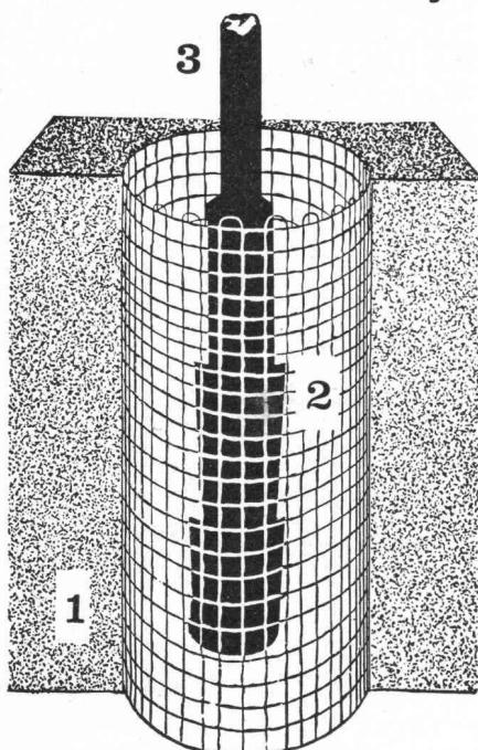
1 = Schnitt Beton    2 = Beton-Drahtkern
