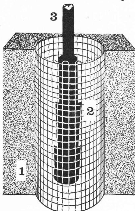
1 = Schnitt Beton    2 = Beton-Drahtkern
