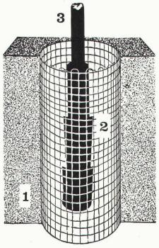
1 = Schnitt Beton 2 = Beton-Drahtkern
