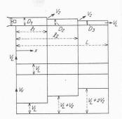
$$\frac{V_L + 2V_Z}{D_1^2} = \frac{V_L + V_Z}{D_2^2} = \frac{V_L}{D_3^2} = \text{konst}$$
