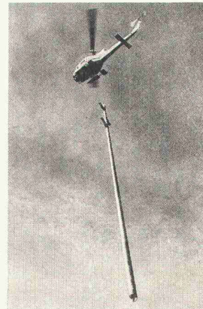
Transport eines 26-m-Mastes
